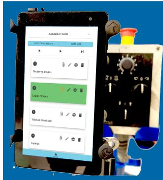
Programmable control system for newfiro piece positioner equipment
